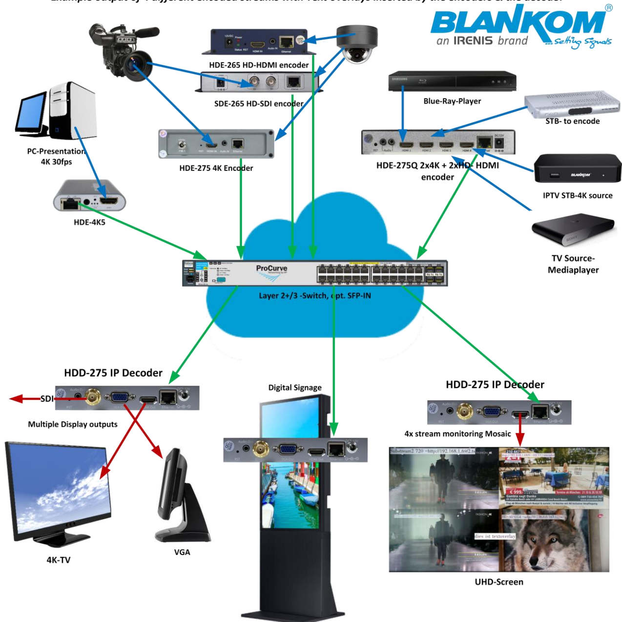
Example output of 4 different encoded streams with Text overlays inserted by the encoders & the decoder
