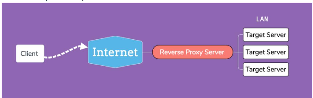
FRP is a fast reverse proxy to help you expose a local server behind a NAT or firewall to the internet. As of now, it supports tcp & udp, as well as http and https protocols, where requests can be forwarded to internal services by domain name.
